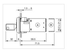
$\label{eq:approx} \begin{array}{l} A = Screw \ terminal \\ B = Plug-in \ terminal \ 6.3 \ mm \ x \ 0.8 \ mm \end{array}$
