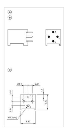
A = Axial socket B = Occupancy plan (component side) C = Drilling plan (component side)
